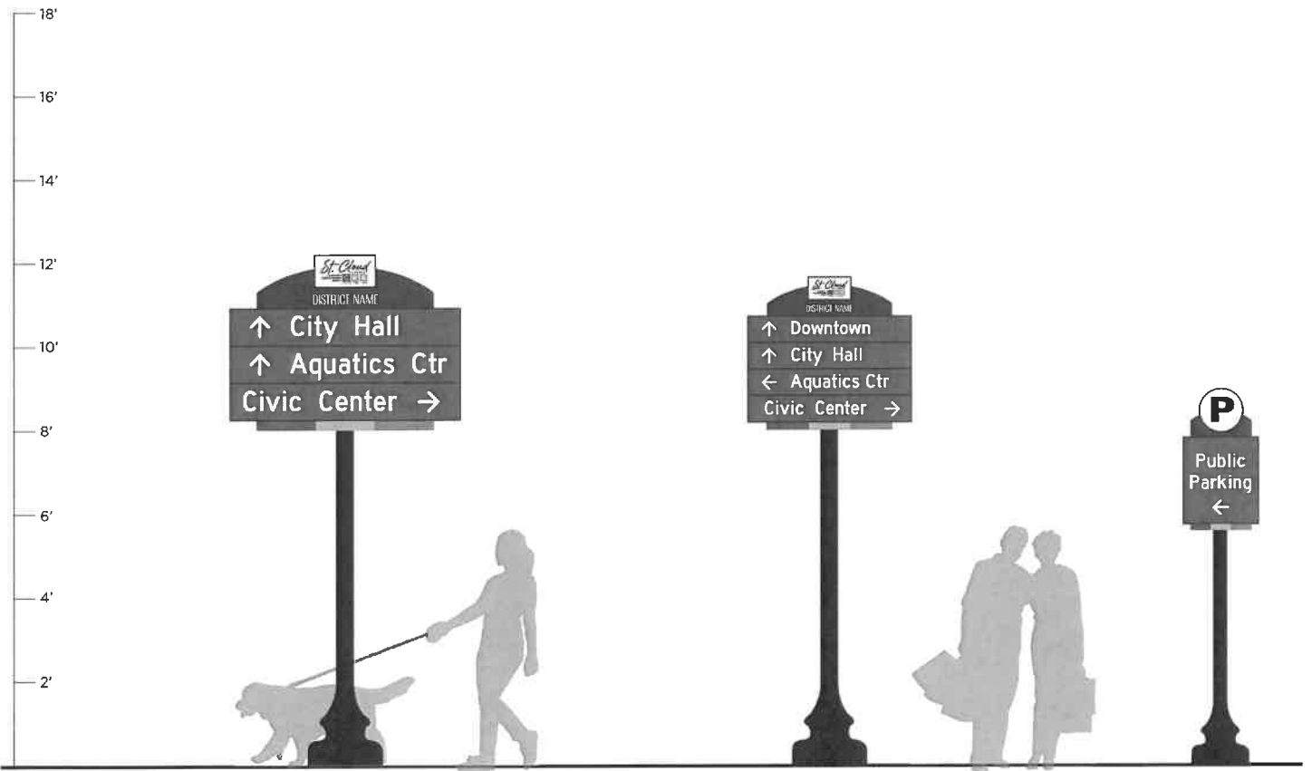
B Large Vehicular Sign (FDOT roads)
